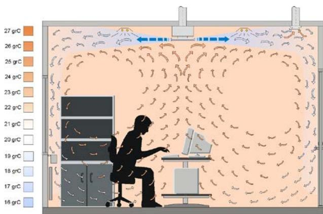
Figure 2. Vertically displacement ventilation. The inlet-air is supplied via air showers and does not disturb the convection currents from the heat loads in the room
